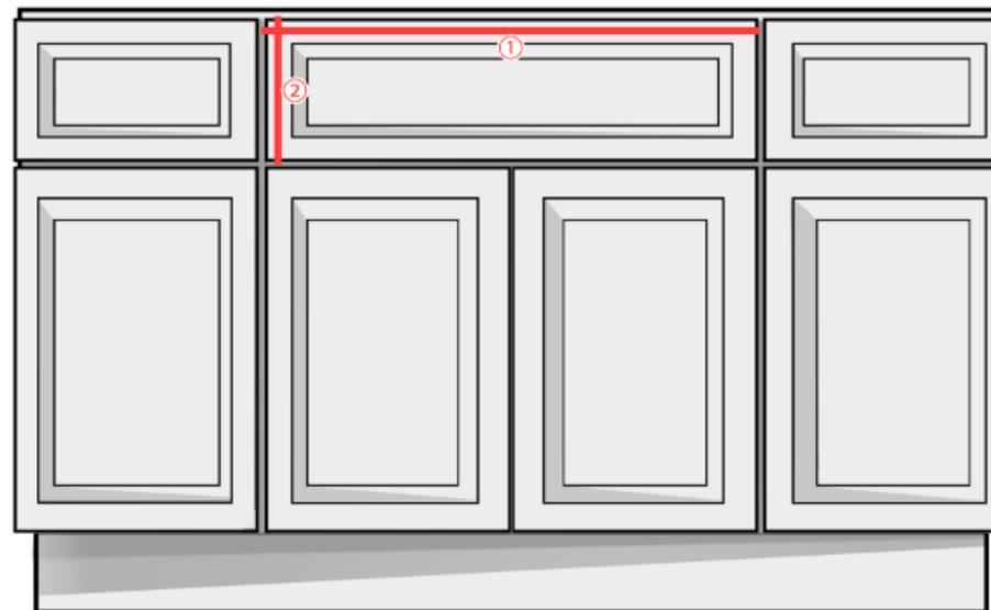
**INSTALLATION NOTE:** THE APRON LINES UP WITH THE DOORS BELOW AND WITH THE ADJACENT DRAWERS. THERE IS A 1 INCH CHANNEL BEHIND THE APRON THAT SIMPLY SLIPS OVER THE FACE FRAME OF THE CABINET ONCE THE FALSE DRAWER HEAD OR HEADS ARE REMOVED.
