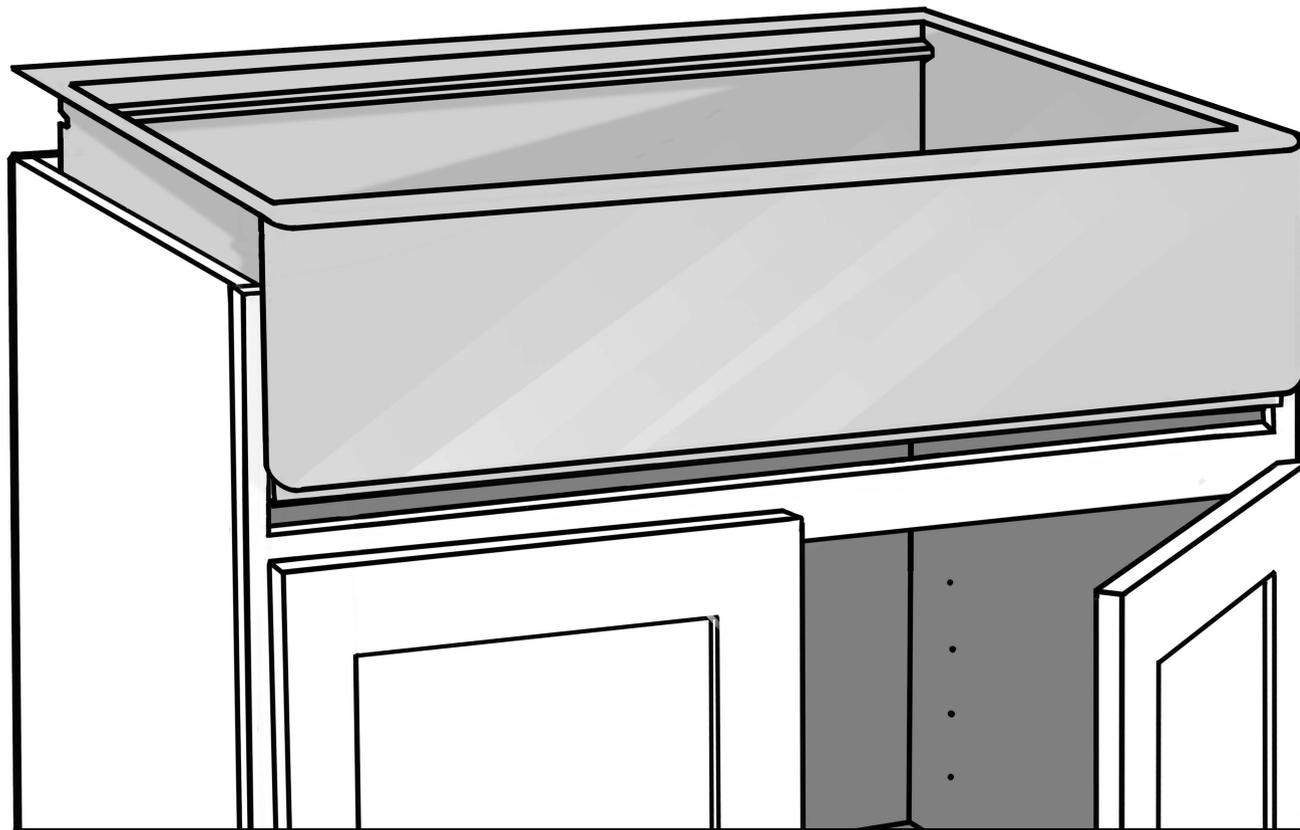
**INSTALLATION NOTE:** THE APRON LINES UP WITH THE DOORS BELOW AND WITH THE ADJACENT DRAWERS. FOR UNDER-MOUNT SINKS, THE COUNTER TOP SHOULD BE CUT TO SIZE WITH THE SINK INTERIOR, AND INSTALLED WITH NO OVERHANG, AND NO REVEAL.
