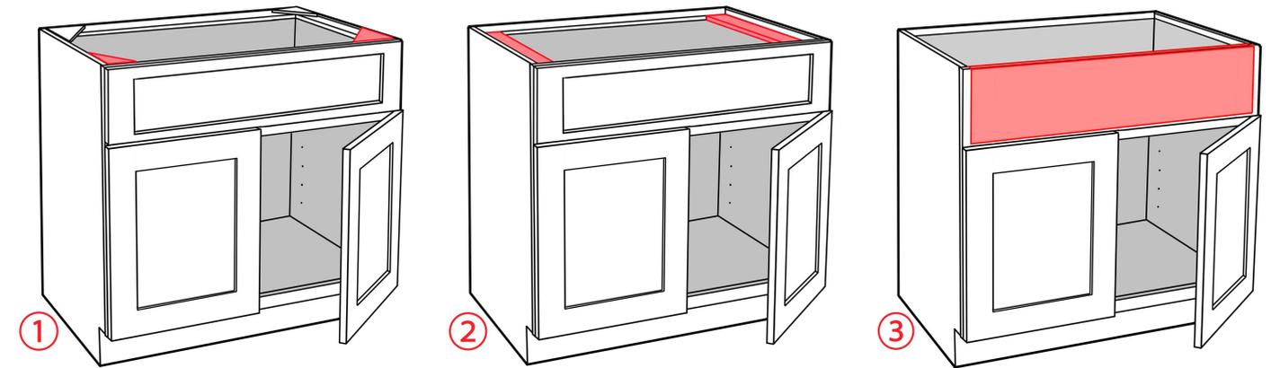
FIRST, DEPENDING ON YOUR CABINET DESIGN YOU'LL NEED TO REMOVE EITHER THE FOWARD **CORNER GUSSETS** ① OR LEFT AND RIGHT **SIDE SUPPORTS** ② FROM THE TOP OF YOUR CABINET OPENING. THIS WILL ALLOW THE SPACE NEEDED FOR YOUR SINK BOWL TO INSTALL SMOOTHLY AND WITHOUT OBSTRUCTION.
